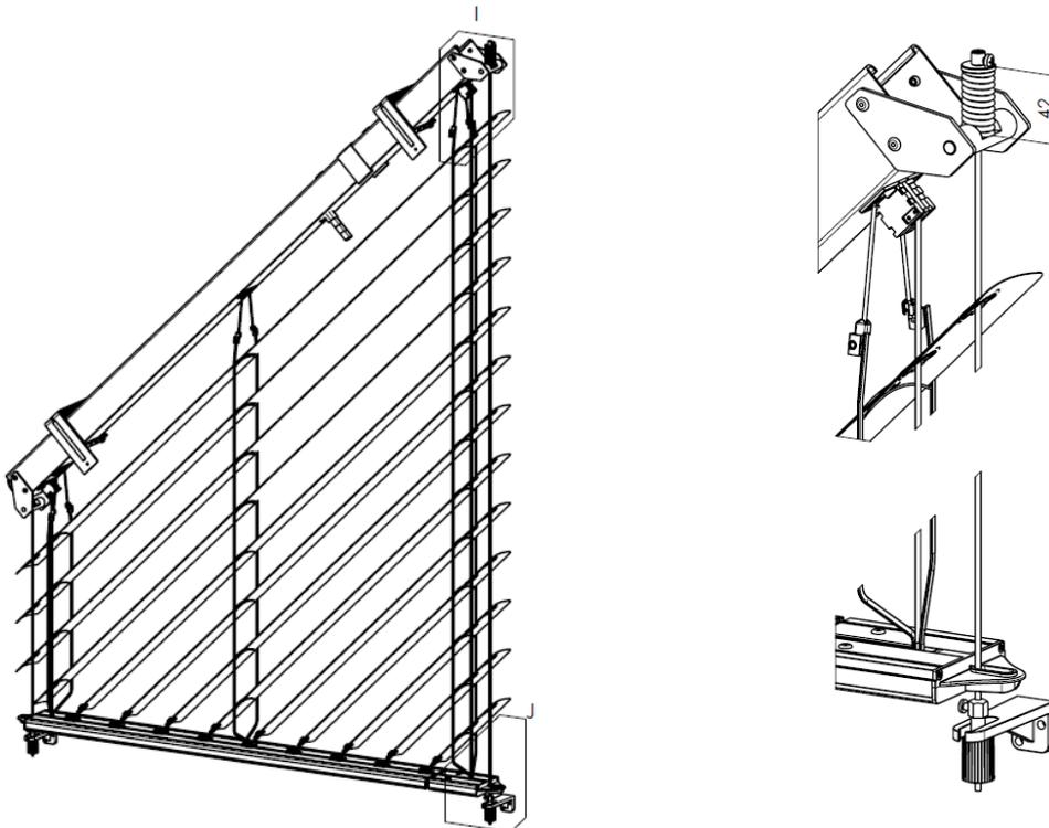
Using sloped blinds it is necessary to achieve correct wire tension to avoid its big undesirable sag while retracting the blind.
