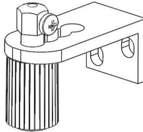
1. After choosing the correct position of wire guiding bracket and its screwing it is necessary to release the plastic housing with female screw up to edge of the tensioning screw thread (unscrew).
